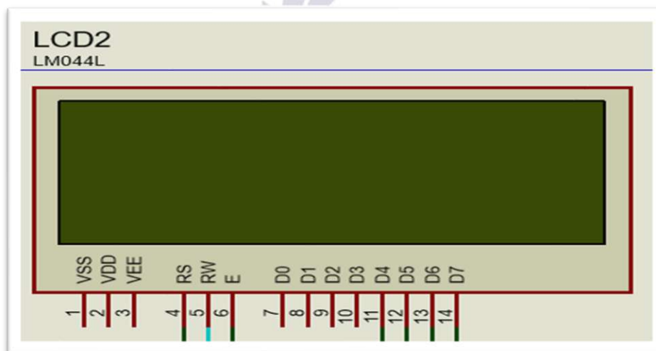
Figure 01: 16x4 LCD Display Schematics
