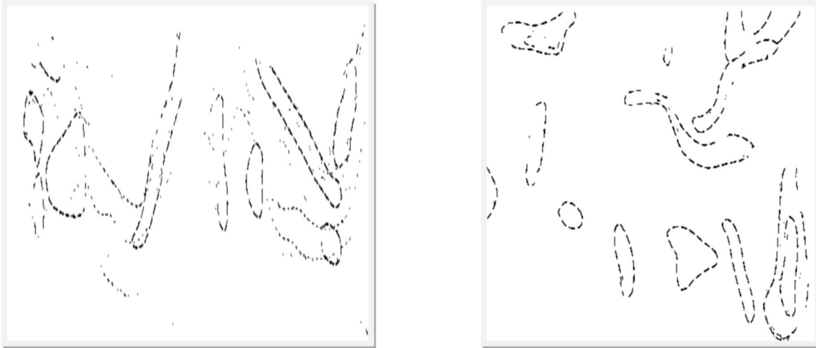
Figure 8: Extraction of Dash Line Pattern by Proposed CNN from Complex Meteorological Map
