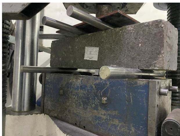
Figure 29 Point load beam test for 28 days cured specimen
