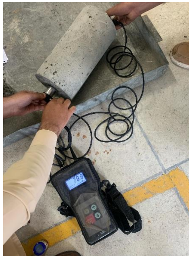
Figure 30 UPV test performed on 14 days cured specimens
