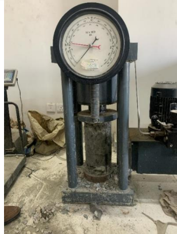
Figure 12 Compressive strength Of 5% RHA concrete specimen
