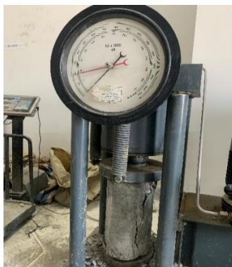
Figure 15 Compressive strength of 15% RHA concrete specimen
