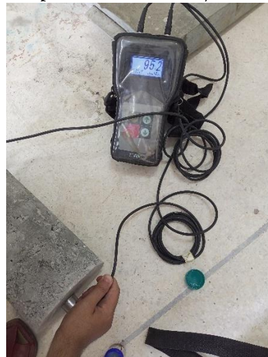
Figure 32 UPV test performed on 28 days cured specimens with 2.5% RHA
