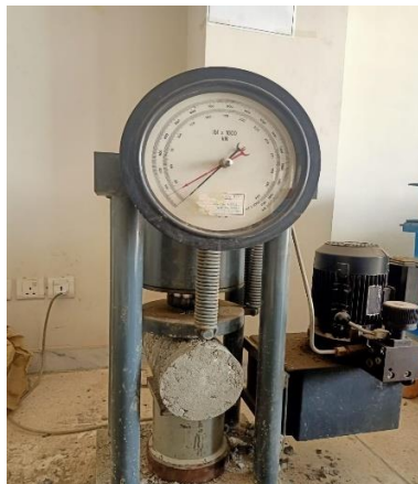
Figure 17 Split Tensile strength of 2.5% RHA concrete specimen
