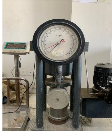
Figure 27 Split Tensile strength of 15% RHA concrete specimen
