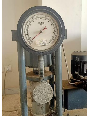
Figure 16 Split Tensile strength of Plain cement concrete specimen
