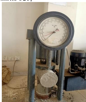
Figure 18 Split Tensile strength of 5% RHA concrete specimen
