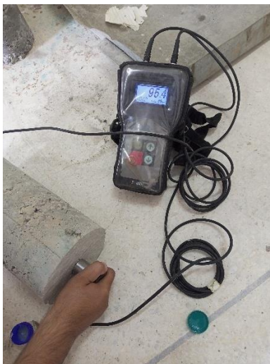
Figure 34 UPV test performed on 28 days cured specimens with 7.5% RHA
