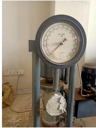
Figure 21 Split Tensile strength of 15% RHA concrete specimen
