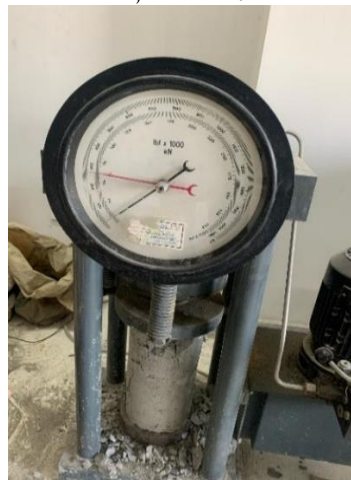
Figure 14 Compressive strength of 10% RHA concrete specimen
