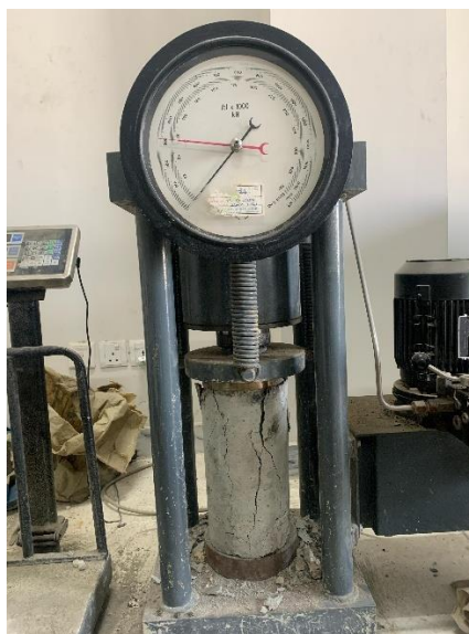
Figure 10 Compressive strength of PCC
