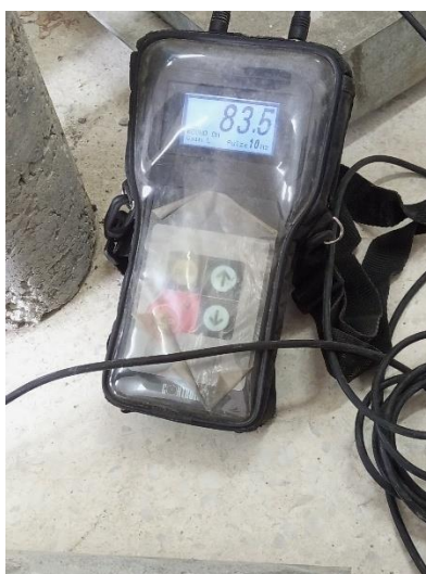
Figure 35 UPV test performed on 28 days cured specimens with 10% RHA
