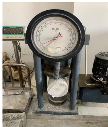
Figure 25 Split Tensile strength of 7.5% RHA concrete specimen
