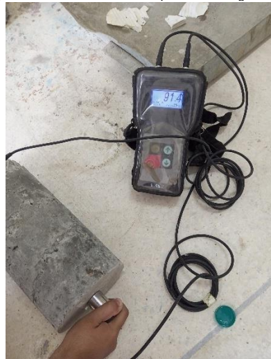
Figure 32 UPV test performed on 28 days cured specimens with 2.5% RHA
