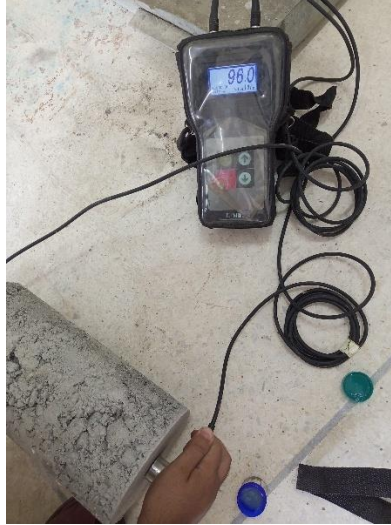
Figure 31 UPV test performed on 28 days cured PCC specimens
