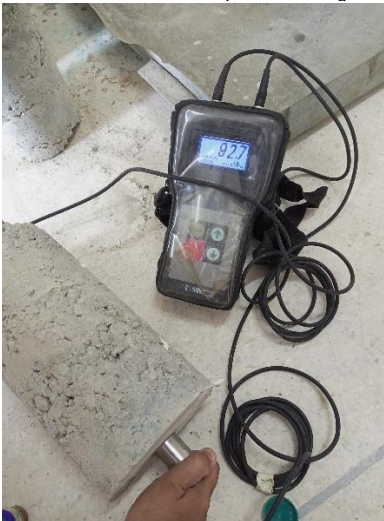
Figure 35 UPV test performed on 28 days cured specimens with 10% RHA
