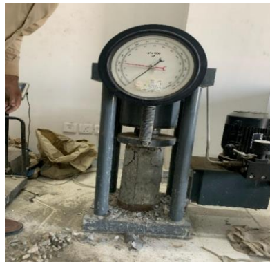
Figure 13 Compressive strength Of 7.5% RHA concrete specimen
