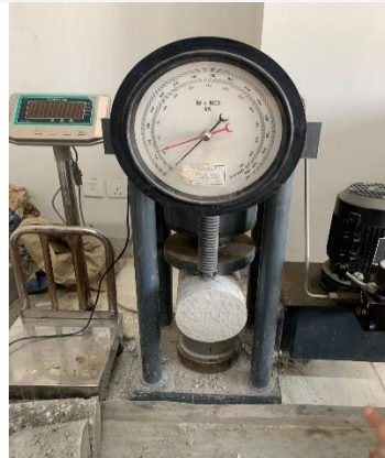
Figure 24 Split Tensile strength of 5% RHA concrete specimen
