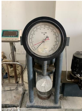
Figure 22 Split Tensile strength of Plain cement concrete specimen
