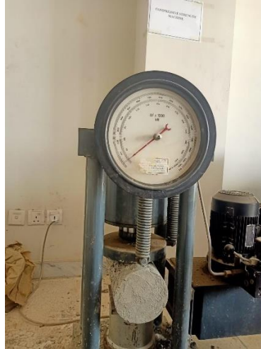
Figure 19 Split Tensile strength of 7.5% RHA concrete specimen
