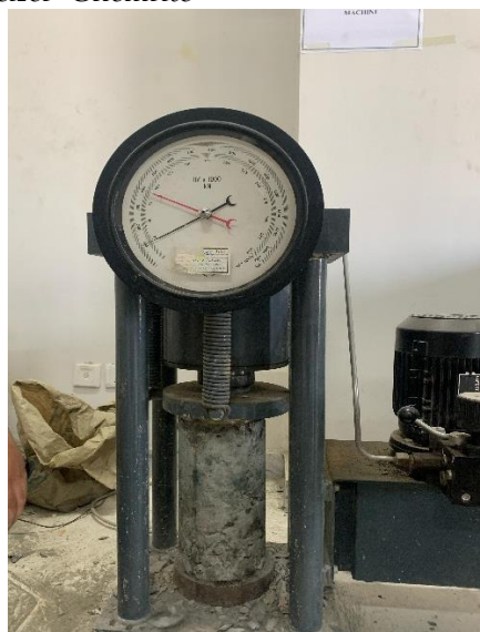
Figure 11 Compressive strength of 2.5% RHA specimen
