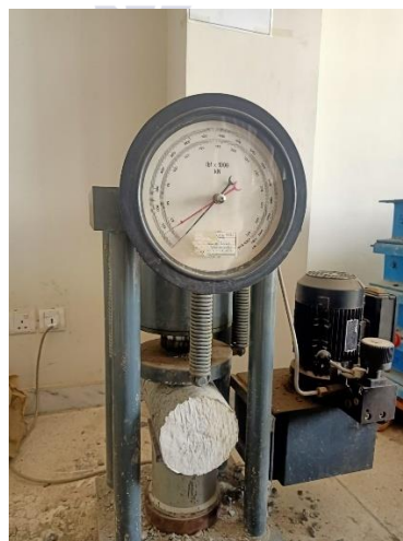
Figure 20 Split Tensile strength of 10% RHA concrete specimen
