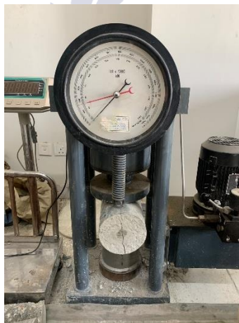
Figure 23 Split Tensile strength of 2.5% RHA concrete specimen
