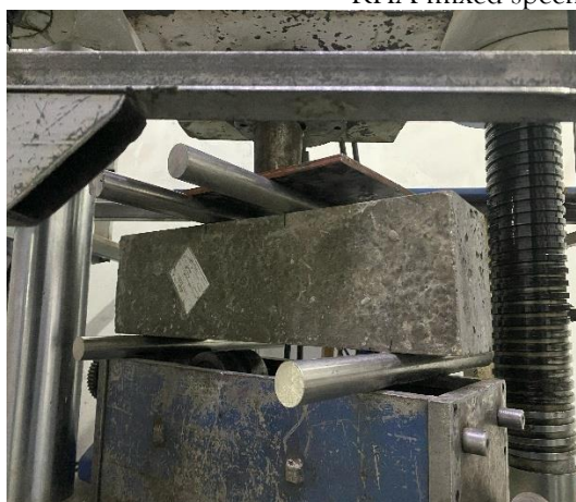
Figure 28 Point load beam test for 14 days cured specimen
